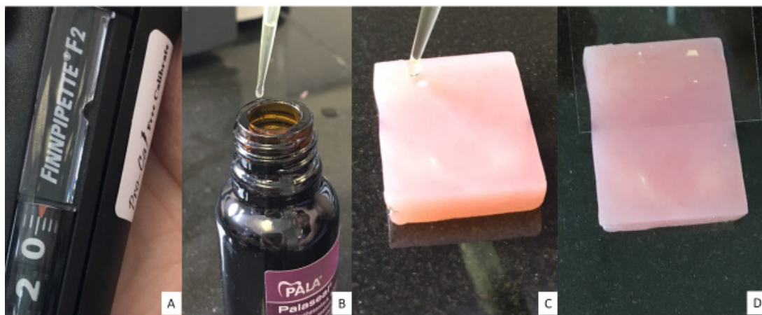
Figure 1 Procedures of Palaseal® coating. A: set a measurable micropipette at 20 µl., B: take Palaseal® with the micropipette tip, C: drop it on prepared PMMA specimens, D: put a cover slide sheet on the specimens and polymerize the specimens with light curing HiLite® power unit for 90 seconds after an exposure time approximately 20 seconds.
