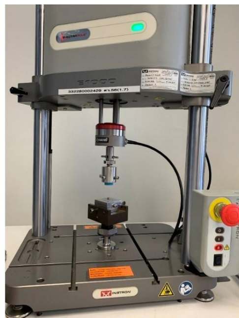
Figure 4 Samples and Instron Universal Testing Machine (e1000, England)
