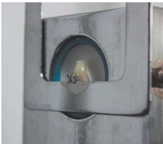
Fig. 2 The apparatus assembled for testing shear bond strength
