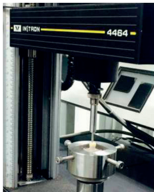
Figure 4 The load application in the central fossa with a 4 mm diameter stainless steel indenter
