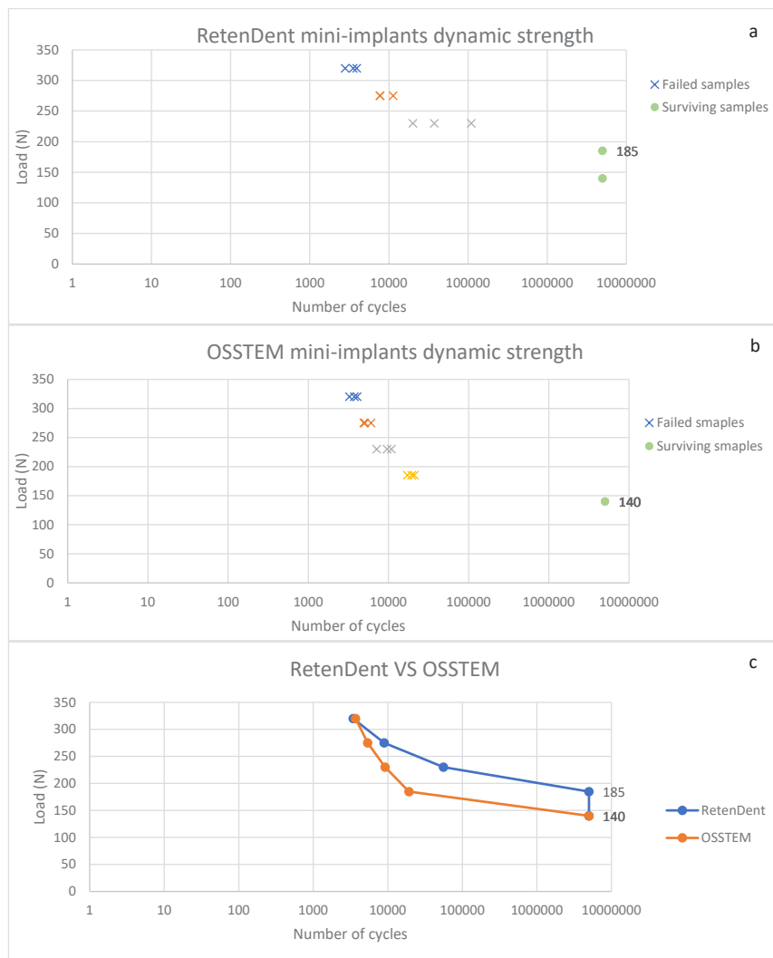
Figure 3 Load-cycle diagram a: RetenDent b: OSSTEM c: RetenDent compare to OSSTEM mini-implant
