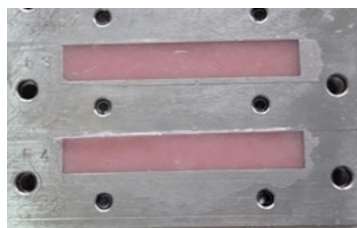
Figure 1 Stainless steel mold with loaded material
