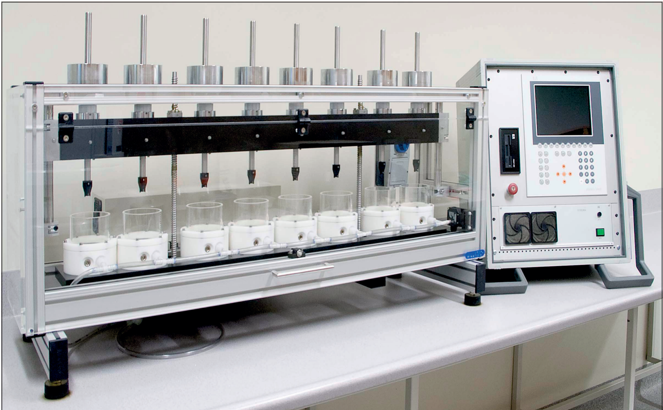
Figure 2 The Willytec dual-axis Chewing Simulator
